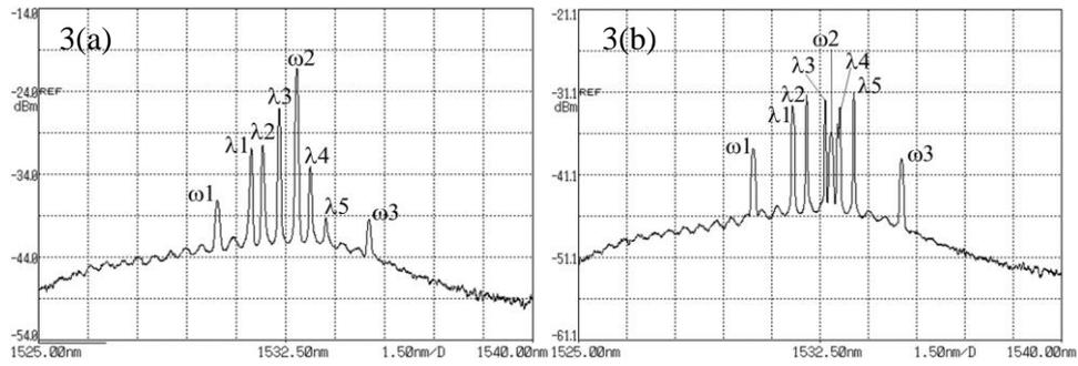
**Fig. 1.** EDFRL generated spectrum which produced multi wavelength through the experimental setup with PCF ZDW at (a) 1550 nm and (b) 1040 nm
