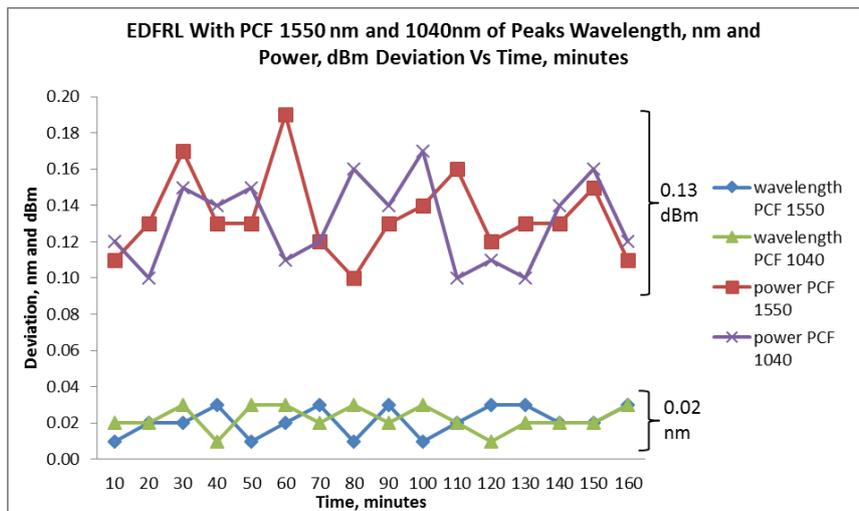
**Fig. 2.** Peaks wavelength and power deviation output based on 160 minutes duration
